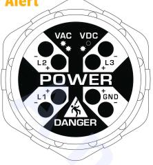
The UPA-100 Power Alert reduces the risk of electrical arc flash by pre-verifying the electrical isolation from outside of a control panel. Hard wired to the circuit breaker or main disconnect, the UPA flashes whenever voltage is present. Engineered with redundant circuitry, the Power Alert is powered by the same voltage that it indicates.
