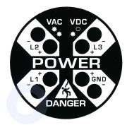
The UPA-130 Power Alert reduces the risk of electrical arc flash by pre-verifying the electrical isolation from outside of a control panel. Hard wired to the circuit breaker or main disconnect, the UPA flashes whenever voltage is present. Engineered with redundant circuitry, the Power Alert is powered by the same voltage that it indicates.
