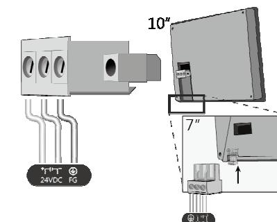
To make a connection, strip about 3/8" of insulation off the end of the wire, turn the connector screw counterclockwise until the gap is wide open, insert the wire all the way in, and turn the screw clockwise until it's tight.
