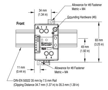
Clearance for Air Flow and Bending Radius 26 mm 102 mm Side (1.03 in) (4.00 in) 40 mm (1.56 in) 94 mm 71 mm (2.80 in) (3.69 in) 41 mm (1.60 in) Rail Release Tab 102 mm (Pull Down) (4.00 in) Clearance for Air Flow and Bending Radius Zero Electrical Clearance Required
