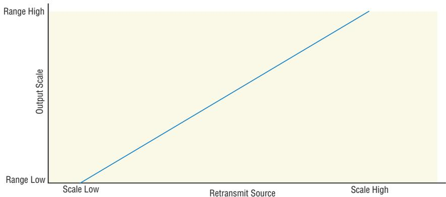
Set the range of the process output with Scale Low  and Scale High . Scale the retransmit source to the process output with Range Low  and Range High .
